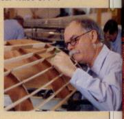
Daycleth "Doc" Walker, whom you met in February *Pilot* ("AOPA Centennial of Flight Sweepstakes: We Have Wings!"), is putting a wood-slat cage on the steel-tube fuselage. The covering will be fastened to it. Dan Pfleger is rebuilding the rudder. Tom Novak is working on the trim systems.
